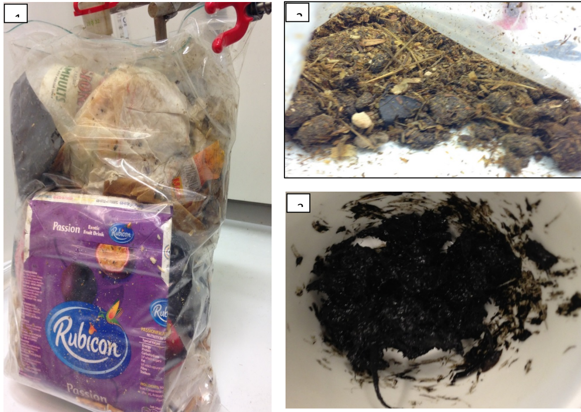
Figure 1: Pictures of the biomass samples (as received): 1- mixed MSW, 2-horse manure, 3- household waste sludge.
